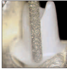
Fig 45 Refining the milled geometric design using diamond-tipped burs and jets of water and air to prevent overheating, which could damage the abutment's structural integrity. (Photographed with a Zeiss OPMI 19-FC stereomicroscope; magnification \times 6 .)
