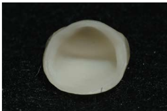
Figure 13: Well etched, clean, internal surface after removal of white precipitate. Compare to Figure 11
