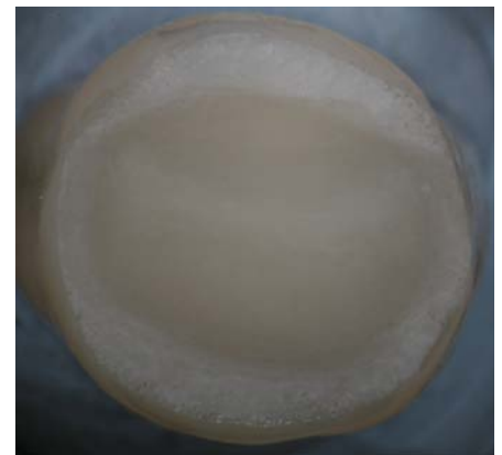
Fig. 23 Etched, uncontaminated internal surface of crown ready for bonding
